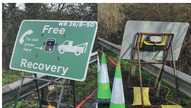
The CCT can also be deployed as an emergency call point for road users to summon vehicle recovery services. Having an accident or breakdown in the middle of road works can be a worrying time so having a readily accessible emergency call point provides vital comfort and reassurance to road users. At the push of a button, they can speak with someone, explain their emergency situation and get reassurance that help is on its way.
