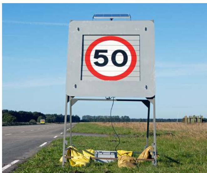
Dynamic Speed Signs have changed this. Using digital technology, the new signs can automatically change to display 40, 50 or 60 mph according to the works programme. This removes the need for operatives to physically change signs which keeps them safe. It also allows traffic to flow freely at 60 mph when works are stopped, minimising disruptions and improving journey times.
