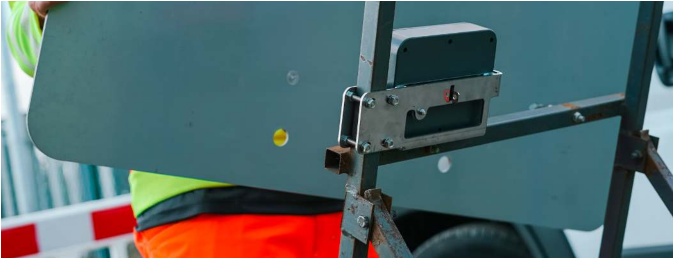
Figure 3. Intelliframe® Lite can be retrofitted to existing frame in seconds allowing remote monitoring of their status and plotting them on a map interface
